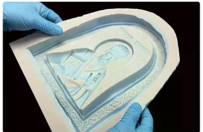
6. Cure and Demold
