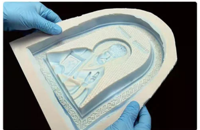
6. Cure and Demold
