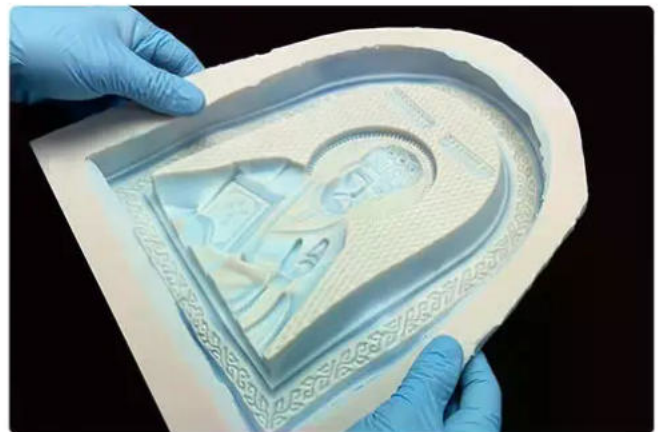
6. Cure and Demold 6. Curar y desmoldar
