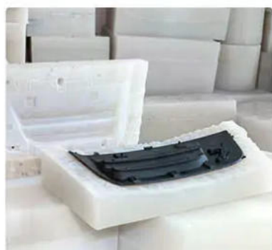
Thin Wall Enclosure Casting 薄壁外殼灌注
